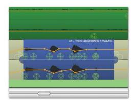
Pan moves can also be created in a Spatialisation window by dragging the mouse around multiple Image Definition objects. Pan trajectories between pairs or groups of Image Definitions can also be entered and edited numerically.
