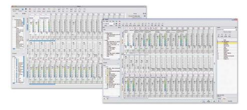
A PC or Mac software suite allows the systems integrator or sound designer to assign all source and zone routing, level and EQ configurations to Presets (Cues).
